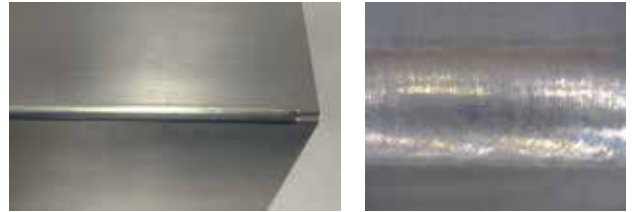
Corner weld on 6061-T6 aluminum (thickness 1.5 mm). The picture on the left showing the overall quality and the microscopic image on the right showing the close up of the weld
