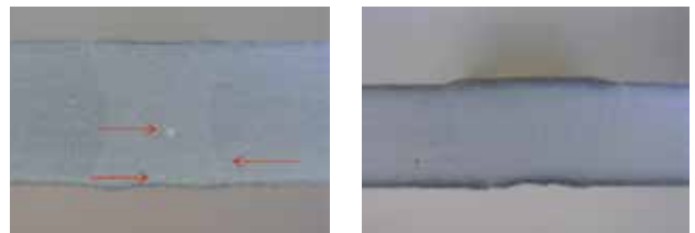
6061 aluminum sample welded with conventional laser welding process: obvious pores in the cross section
