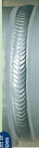
Pulsed current 200A, Base current 20A, Pulse frequency 2Hz AC frequency: 150Hz, Welding speed: 20cm/minute, Plate thickness: 4mm (A6062)
