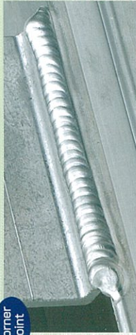
Welding current: 130A, AC frequency: 150Hz Welding speed: 25cm/minute, Plate thickness: 3mm (A6063 + Casting)
